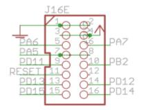
The original J16 functionality is preserved, but extra pins are available on an IDC16 header. These include the Reset signal and pins normally controlling LEDs. This header is normally connected to the RES-SD module.
