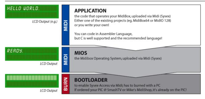
MIOS is the operating system of the microchip. It can be uploaded by SysEx (via MIDI) thanks to a bootstrap loader, a special software that is already burned onto the chip if you order at SmashTV's or Mike's Shop.
