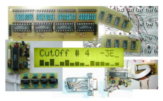
The MIDIbox Hardware Platform is the consequential continuation of my work on MIDI controllers in the last years. It brings down every design to one standardized environment with reusable and exchangeable modules.
