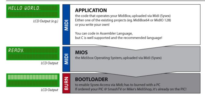
MIOS is the operating system of the microchip. It can be uploaded by SysEx (via MIDI) thanks to a bootloader, a special software that is already burned onto the chip if you order at SmashTV's or Mike's Shop.
