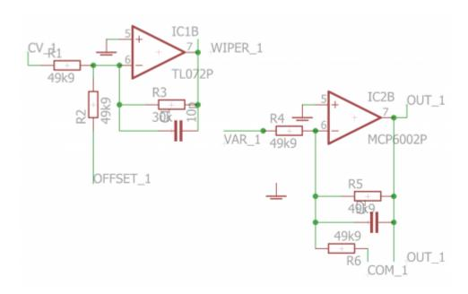
The circuit is a very simple series of two inverting amplifiers per channel. The first is a TL072 powered from  $\pm 12/-12V$ , while the second is an MCP6002 powered from  $\pm 3v3/0V$  (ground). It's possible to preset the ranges (see below) but it's probably more useful to use the associated Control Board.
