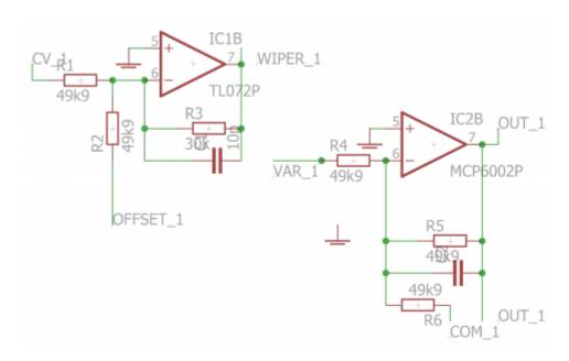
The circuit is a very simple series of two inverting amplifiers per channel. The first is a TL072 powered from +12/-12V, while the second is an MCP6002 powered from 3v3/0V (ground). It's possible to preset the ranges (see below) but it's probably more useful to use the associated Control Board.
