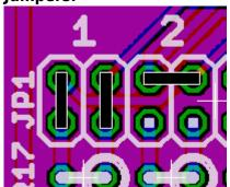
By setting jumpers on JP1 and JP2, you can select normal or bipolar operation for each CV channel. When setting two jumpers like on channel 1 of the picture above, the channel is in bipolar mode.
