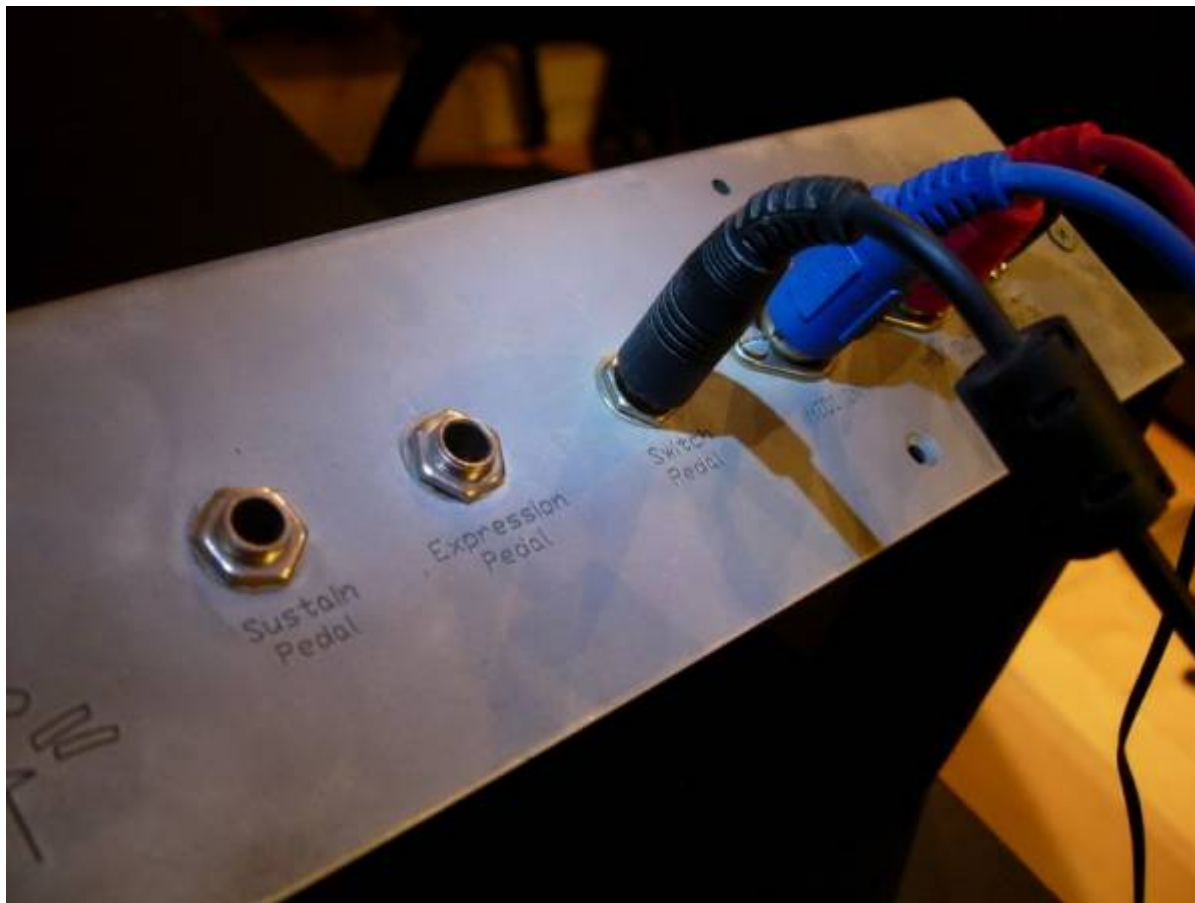
Sustain, expression, and switch pedal inputs; MIDI In/Out, power
