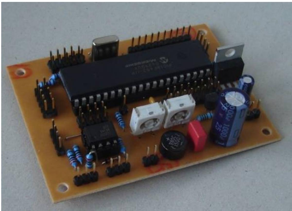
Main part of this module is the PIC, a microcontroller manufactured by Microchip. It is clocked at 40 MHz (externally with a 10 MHz crystal) and offers enough performance to handle analog and digital modules with latencies below 1ms.
