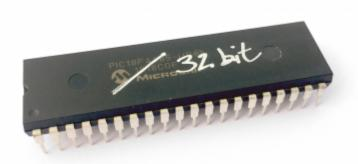
A reduced Core for your MIDIbox App, an STM32F405RG in a DIP40 format.
