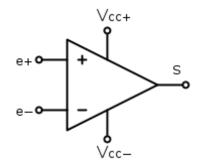
Vcc is the "power supply" voltage for the Operational amplifier
