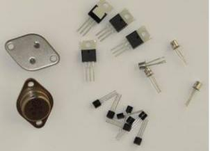
The Transistor is an **active** component that works as an **amplifier** or a **driven switch**.
