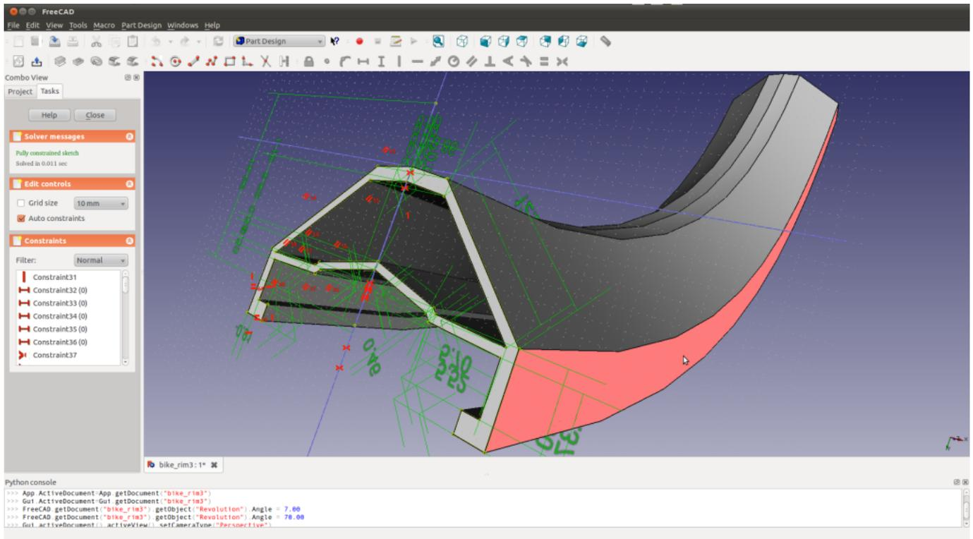
The main feature is its parametric geometry engine and its modifiers pile, overpowered by the OpenCascade library. For those who already know SolidWorks, the GUI is quite designed the same way. It is fully compatible with KiCAD 3D parts, that's why it could be very useful to design cases
