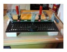
I placed some placeholders (screw with a flat head + metal tube) on the "button-side" of the pcb, put some adhesive on the frontpanel as well and gently placed the pcb on the frontpanel. The buttons and knobs guided the pcb to its right position. The leds are just placed roughly on the pcb before I glued it onto the frontpanel and soldered afterwards.
