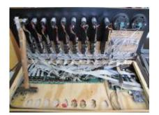
The case is also made out of beech wood. I will post some pictures of how to build one in the next chapter. The small holes you can see on the bottom of the case are for the faders. I wanted the case to be as slim as possible, but I didn't consider the cables coming out of the fadermotors  $\Join$ . I didn't want to redo the whole case (I only have limitied access to a woodshop) so I just cut out some holes.
