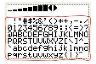
So, at first you need an empty graphic which you're overlaying with guidelines, creating  $8 \times 16$  evenly sized cells. Every cell has to have a height of a multiply of 8 pixels (8, 16, 24, ...).
