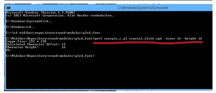
Next to the script name and the name of the file that is to be converted there has to be a parameter "-icons XX" that gives the number of icon columns and the parameter "-height XX" that gives the height of a single icon. The script then calculates the width of the icons.
