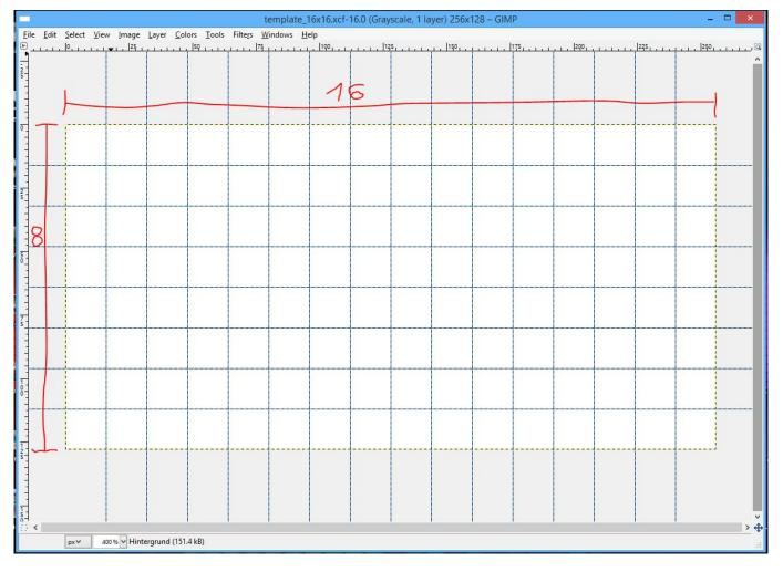
Now you can fill the cells with whatever graphics you like, but only black and white are allowed. In this example I put in a font named "crystal" I found on the web and modified it a bit. Here all the cells have a size of  $12 \times 16$  (WxH) pixels.
