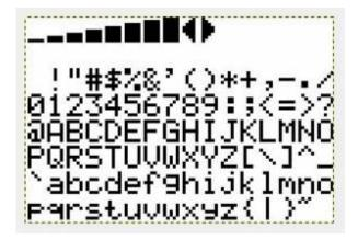
This is an original font file from TK. It consists of 8 rows and 16 columns, that makes 128 cells, so technically 128 icons can be put in. The top row is used for the default bar and some special icons used by the Midibox. The second row is empty for it's not used by the Midibox\_NG firmware (afaik). You could also manipulate the default bar and arrow icons, but I will focus on creating usable icons in the six lower rows.
