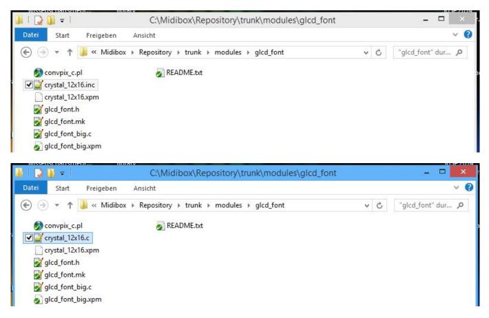
Next you have to open the image file (now "crystal\_12x16.c") with the texteditor and fill in the necessary header information. At line 5 give it a name (case sensitive!) and open a function. At line 6 define the size of the icons and the offset (normally a width of 12 would need a char offset of 12. This means, MIOS is looking after 12 pixels for a new icon).
