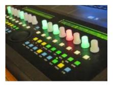
Since I used a custom design I put all the buttons/leds/encoders on a standard 0,1 inch vectorboard. I had to cut a hole into it because I had to fit the data wheel in between.
