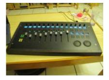
Since I successfully built my SEQv4 I used similar methods when I built the Mackie Clone. All the buttons/encoders/displays are soldered on a standard 0,1 inch pcb. I used a 500mmx100mm pcb and placed 14 of the displays on it. For the remaining 4 displays and the corresponding buttons I had to attach a smaller piece at the lower right side. This piece was a leftover from the SEQv4 pcb.
