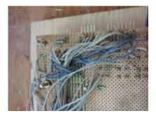
After I finished soldering the pcb I cut out the spaces for the faders. I wanted to save space so I placed the track buttons (for mute/solo/select...) between the faders. This was easier said then done! The pcb material is very sturdy and it took a small drill, a pair of nippers and a pair of tongs to do so without damaging the already soldered parts.
