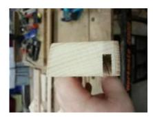
Once all elements are finsihed the 4 fram parts are just mortised, so there are no screws necessary. The baseplate is put in the gap of the frame parts.
