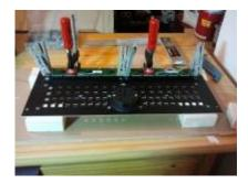
I placed some placeholders (screw with a flat head + metal tube) on the "button-side" of the pcb, put some adhesive on the frontpanel as well and gently placed the pcb on the frontpanel. The buttons and knobs guided the pcb to its right position. The leds are just placed roughly on the pcb before I glued it onto the frontpanel and soldered afterwards.
