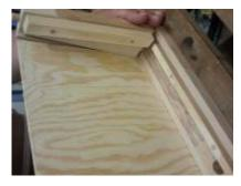
After that all the frame parts get glued with wood glue and helt together with 2 big bar clamps until the glue has dried.
