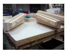
The trick with the baseplate is to cut a gap along the lower bound of the frame parts.
