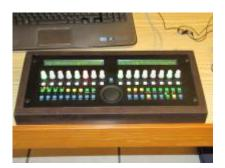
Instead of seperate GP encoders and leds I put in some nice illuminated encoders. They can be connected just like normal encoders and leds, they have seperate pins for each of them.
