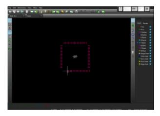
• Lastly, the PCB Design by itself. Based upon your components list and associated footprints, you can create the PCB by placing footprints at the right place and make routing between them (which is connecting components footprints by making copper paths). You can also use the famous 3D viewer to see a simulation of the result.
