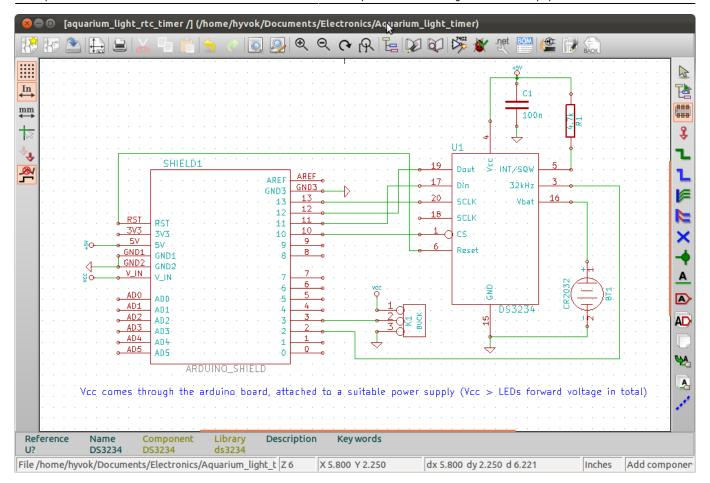
After this you will have to make a link between components and footprints. Footprints are the layouts of pads, holes, and silkscreen drawings that are actually manufactured into the PCB, corresponding to each component.
