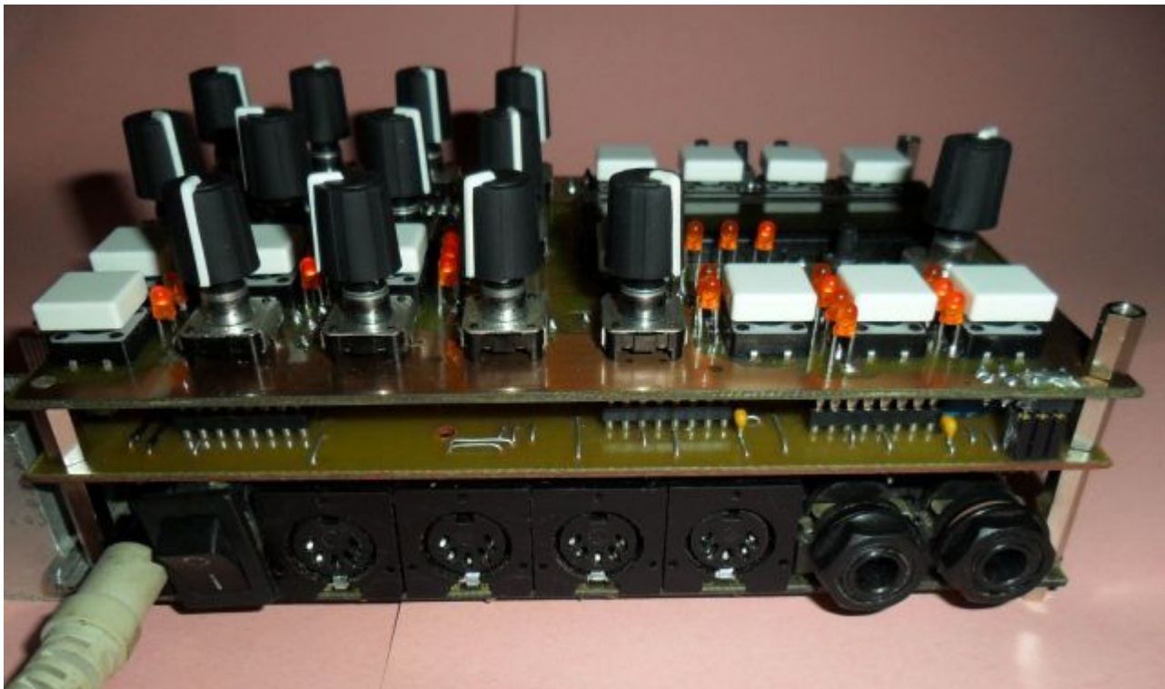
Midibox TWINSid is a light midibox sid v2 on three pcb wiht only two sid chip for stereo
