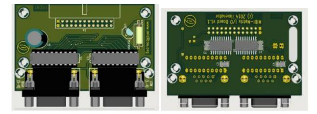
The overall size of the PCB is 50mm x 80mm.
