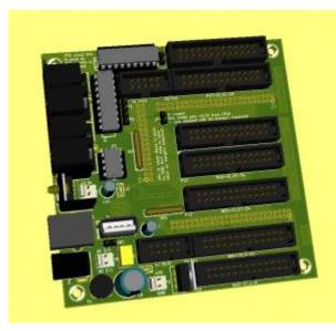
On the left is a rendering of the FPGA board created with KiCAD. This is the second generation v1.1 FPGA board which has a pair of MIDI I/Os, and an AC power plug (which can also be used to feed DC power). The board can loop through the USB signals from the Micro USB plug found on the STM32F4 Discovery board to the outside world when the whole unit is mounted in an enclosure. The FPGA board connects to J8/J9 of the core board for DIN and DOUT chains, and to J11E for MIDI connectivity.
