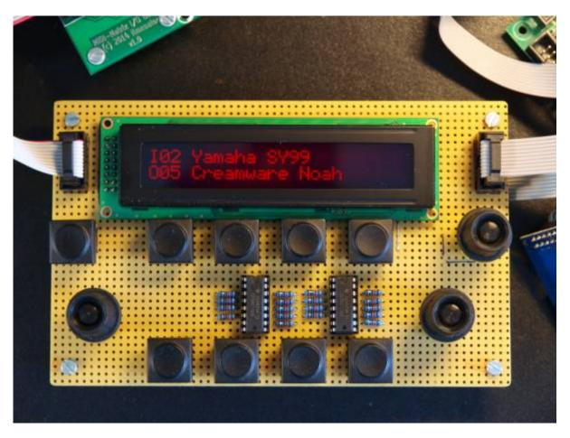
The prototype of the user interface (UI) already shows the main usage paradigm: a rotary encoder (on the lower right) is used to select the out port, thereafter the in port is selected with the rotary encoder on the left. This selection is confirmed by pressing the encoder. More changes to the current routing can be made, and when pressing the lower right rotary encoder, all changes are made effective and the routing is changed.
