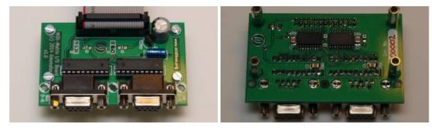
Each I/O Board handles 8 MIDI ins and 8 MIDI outs, i.e. it can connect to up to two BOBs.
