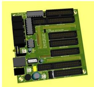
On the left is a rendering of the FPGA board created with KiCAD. This is the second generation v1.1 FPGA board which has a pair of MIDI I/Os, and an AC power plug (which can also be used to feed DC power). The board can loop through the USB signals from the Micro USB plug found on the STM32F4 Discovery board to the outside world when the whole unit is mounted in an enclosure. The FPGA board connects to J8/J9 of the core board for DIN and DOUT chains, and to J11E for MIDI connectivity.
