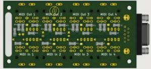
The total size of the PCB is 100mm x 50mm.
