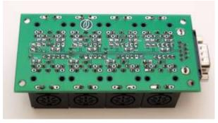
Because I like the idea of recycling components that have barely been used in other, now obsolete equipment, the MIDI sockets can also be replaced with DIN sockets bearing different kinds of footprints and/or additional pins. I frequently use 8-pin DIN sockets de-soldered from old video equipment as they are fully compatible with the 5-pin MIDI plugs. Of course, the standard 5-pin MIDI socket footprint will fit here as well!
