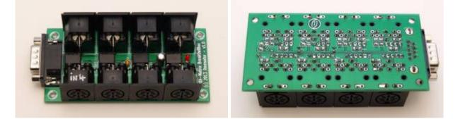
Because I like the idea of recycling components that have barely been used in other, now obsolete equipment, the MIDI sockets can also be replaced with DIN sockets bearing different kinds of footprints and/or additional pins. I frequently use 8-pin DIN sockets de-soldered from old video equipment as they are fully compatible with the 5-pin MIDI plugs. Of course, the standard 5-pin MIDI socket footprint will fit here as well!
