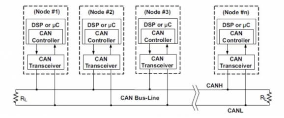
For both connection models, each Node(Device) connected to the buss can transmit or receive data. How is this possible?
