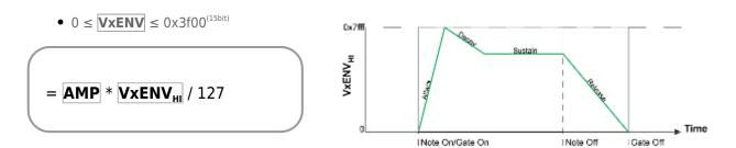
Envelope to Amplitude Enabler in Vx Mode Controller:
