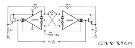
A floating VCR where each "end" of the "resistor" may be at any voltage within the output voltage range of the LM13700.
