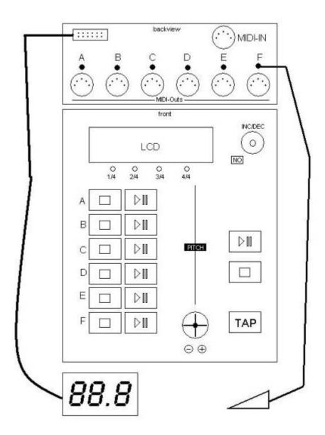
On the top of the picture you can find the backview (jackview). In the middle the frontpanel and on the bottom the peripherie.
