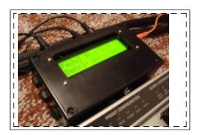
Is an expression pedal controller to expand an existing floorboard. In addition to adding up to 8 expression pedals, up to 8 relays can be triggered and the LCD display reflects the actions of your existing floorboard as well.
