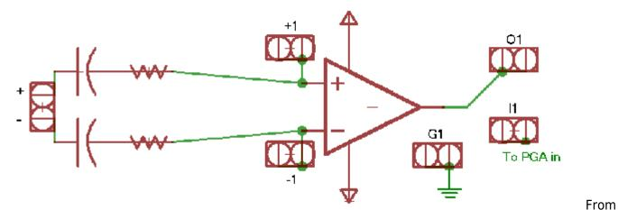
that you can make a LOT of different input sections. A VERY simple input section would be the Unity gain unbalanced input buffer. It's very simple, and looks like this:
