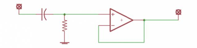
Figuring this out shouldn't be too tough. We follow the input from the "+" input terminal through capacitor C11. We don't need a series resistor here, so we add a wire for the bottom resistor beside C12. We do need a 10K resistor from the + input of the op-amp to ground, so we add it, between the "+1" and "G1" terminals. Then, for the feedback loop, we add a jumper from "O1" to "-1", finally, we connect "O1" to "I1" to pass the result to the PGA input.
