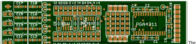
parts needed are: 1 PGA4311 4 channel audio volume control 5 Capacitors, 0.1uf 1 Capacitor, 1.0uf 17 Stack pins
