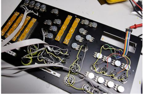
The shot above shows the DIN (pushbutton) wiring completed. I've left the ribbon cabling long until I can determine how long the runs will need to be to get to the modules.
