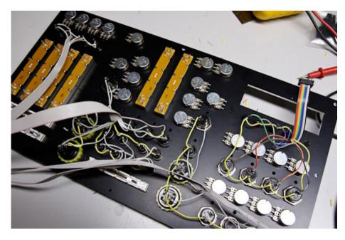
The shot above shows the DIN (pushbutton) wiring completed. I've left the ribbon cabling long until I can determine how long the runs will need to be to get to the modules.
