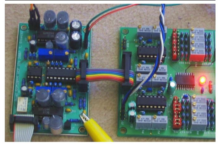
As you can see, on my prototype I didn't take the size of 10nF Styroflex caps into account... New board size is 90x60mm instead of 80x50mm.
