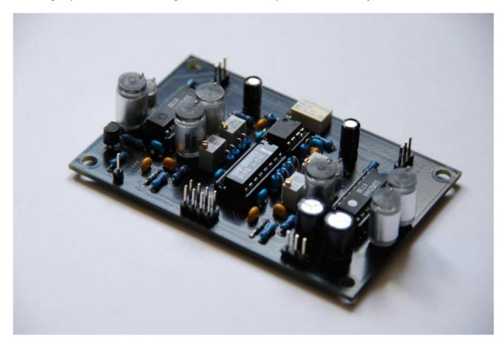
This PCB contains two of the famous SSM2044 24dB low pass filters with the necessary circuitry, additional LM13700 based Q linearization circuit and a tiny Omron micro relay for a software controlled (via gate out pins) bypass function. The layout is optimized for use with the AOUT\_NG module, requiring the addition of a bipolar option when used with regular V/Oct sources like the original AOUT module.
