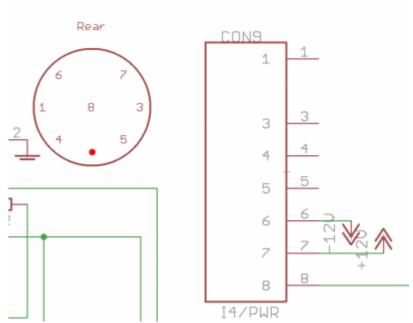
Connector 14. Pin 8 can be connected to +5V or to a higher voltage for downstream regulation.
