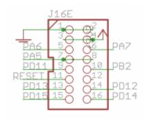
The original J16 functionality is preserved, but extra pins are available on an IDC16 header. These include the Reset signal and pins normally controlling LEDs. This header is normally connected to the RES-SD module.
