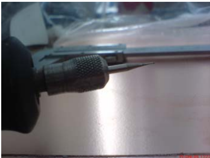
Cutting the new PCB using a small cutter for my dremel tool. Two boards are done, one for the left and the right side of the unit.
