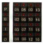
The User-Interface panel consists of 20 buttons. There are 4 "screen-buttons" and 16 "value-buttons".
