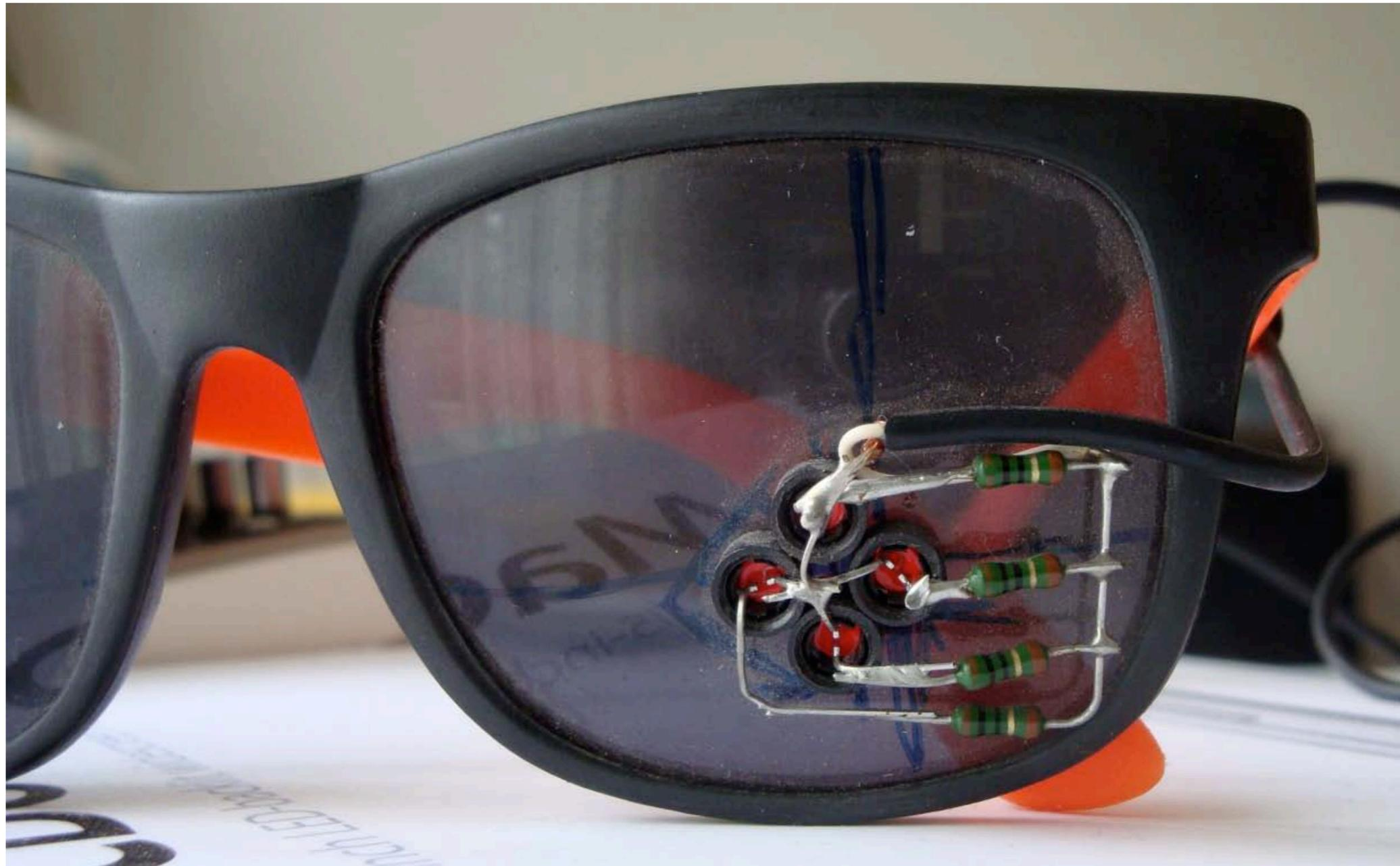
This is how the LEDs are mounted in the \$1 sun-glasses. To find the position of the LEDs, lie down comfortably, wear the goggles (and ear-phones), close your eyes and look straight. Place the LEDs in direct sight.
