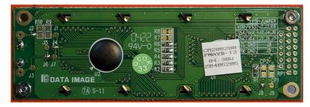
You can also check if the LCD's PCB edge is parallel with the edges of the ground plane gap of the control surface's PCB (i.e. the darker red shape on the bottom which is the exact size of the LCD).
