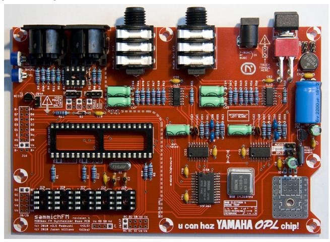
Now is a good time to check for shorts between 5V and GND before you solder the voltage regulator, so you can rule out the voltage regulator as a cause (removing it later is painful!)
