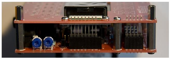
**Step 7.6:** Solder two diagonally opposite pins on each header on the top side, ensuring female header is flat against base PCB.
