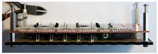
**Step 3.6:** Look underneath at the LEDs and check they all protrude the same amount. If any do not, it could be that a LED is stuck because the hole is slightly smaller or the LED is slightly bigger. Disassemble PCB and panel and check that LED individually. It is possible that a LED has a little bit of excess plastic from molding imperfections, which can be scraped away using a craft knife.
