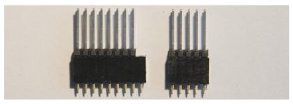
Note: depending on the LCD type, the 16 pin male header goes into the "upper" or "lower" 16 pins of the 18 pin female header. Most of the time it will be the "upper" 16 pins, as shown by the white outline on the base PCB. As far as I know, only the Optrex STEP LCDs require it in the "lower" 16 pins, because the backlight pins are at the other end of the header.
