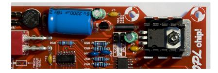
Step 5.3: Place big heatsink onto PCB
