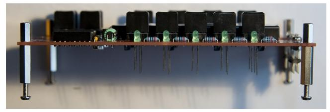
Step 3.4: Attach top panel to PCB using black screws. Check alignment by looking at the switch caps.Step 3.5: Turn PCB upside down. *Carefully and gently* push LEDs into the holes as much as possible.
