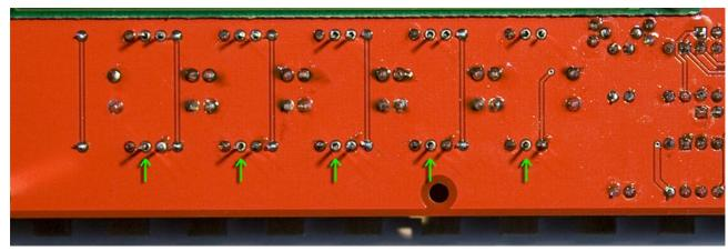
Step 3.9: Solder all the longer leads of that row of LEDs.
