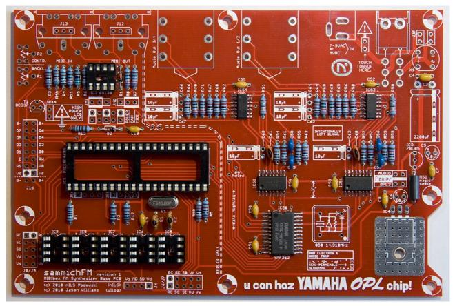
Diodes must be oriented correctly. The stripe on the diode matches the stripe on the part outline.
