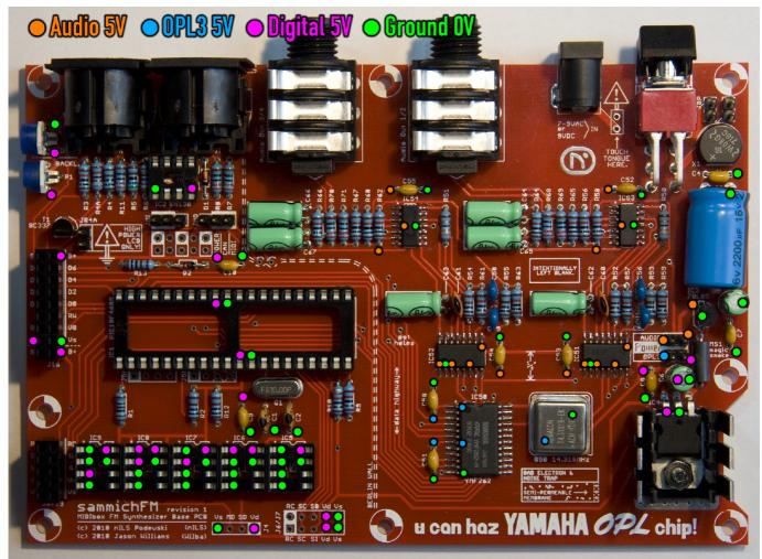
Once you've tested 5V between one pair of pads (such as J4 at bottom), you can leave the black probe on GND at J4 while you test 5V at other points marked with pink dots. Inversely, you can leave the red probe on +5V at J4 while you test for 5V at other points marked with green dots.
