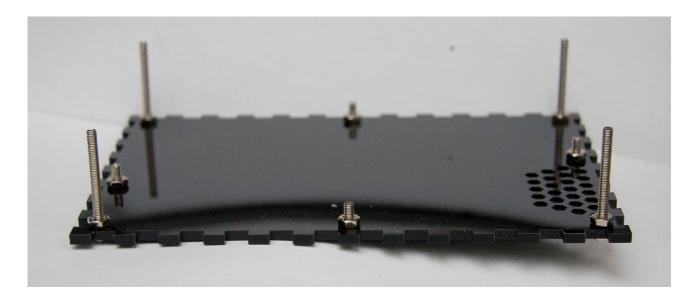
Put the 32mm and 9mm screws into the base panel from the bottom. The 32mm screws go in the corners. Add the nuts and tighten firmly using screwdriver and long-nose pliers.
