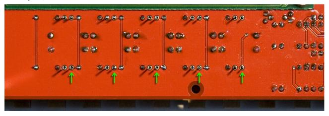
**Step 3.8:** Look underneath at the LEDs and check they all protrude the same amount. If not, heat up a joint and push down on the longer lead (there's a reason I told you to solder the shorter lead first!)
