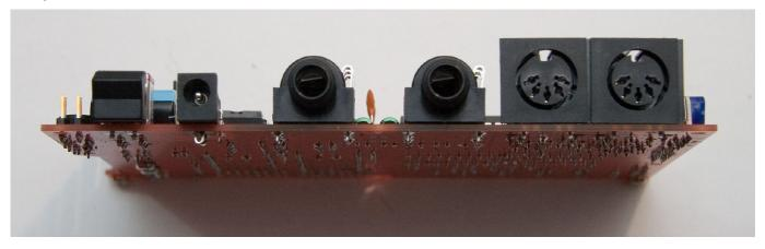
Solder only *one pin* of each socket to hold it in place, then you can check for correct alignment before soldering the other pins.
