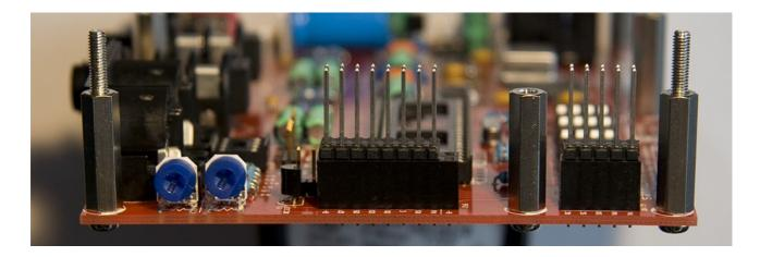
**Step 7.5:** *Slowly and carefully* place control surface PCB onto corner screws and lower down so male header pins go through holes in LCD and control surface PCB. Attach with 10mm spacers at corners and 3mm screws at side midpoints.
