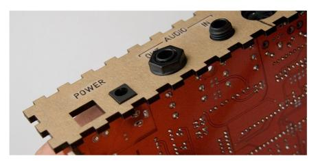
After "tacking" all the sockets, you can now check for correct alignment by placing the PCB onto the base with screws/nuts attached and adding the corner spacers (see **Case Assembly** section) and then attaching the rear panel. You should check that the power socket and audio sockets are not causing the rear panel to have a gap where it joins the bottom panel. If they do, you can heat up the "tacked" joint while you realign the socket.
