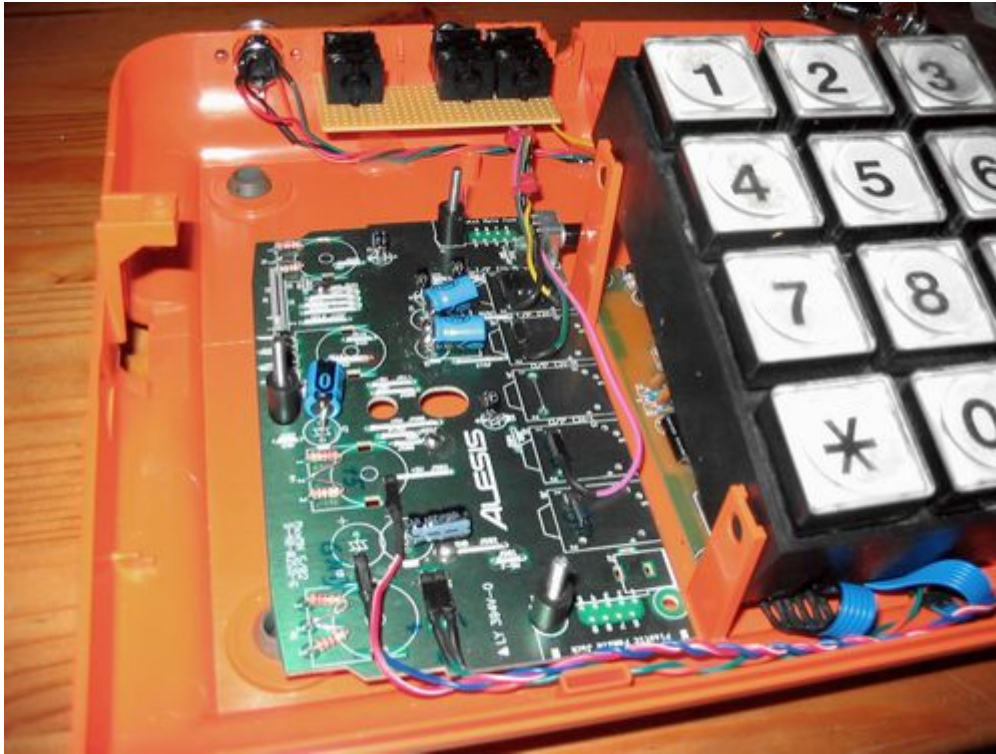
The second board connected. Behind the keypad there's the Sibalance pot.
