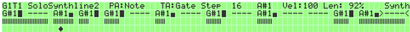
Triggering a glide from step 3 into step 4. The visible layers in the image are note and length parameter layers (first and second), and the glide trigger layer (third).
