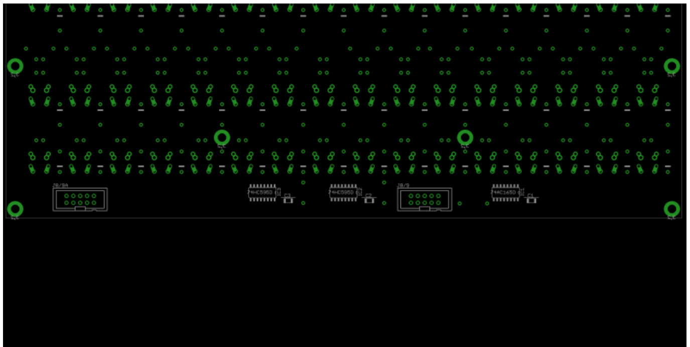
Rear placement of ICs (ignore the "AC" package, the correct CMOS family is 74HC165)
