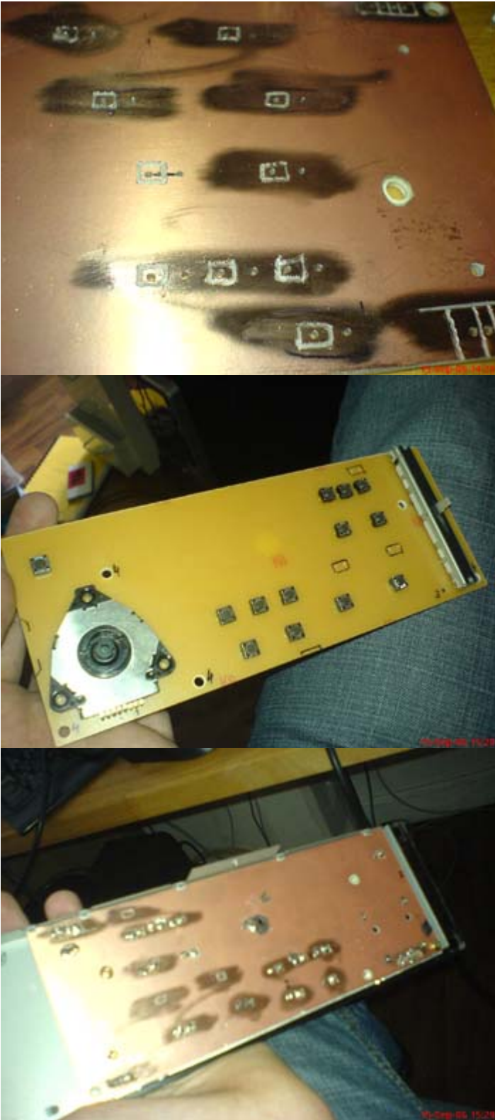
Mounting the parts and attaching cables.
